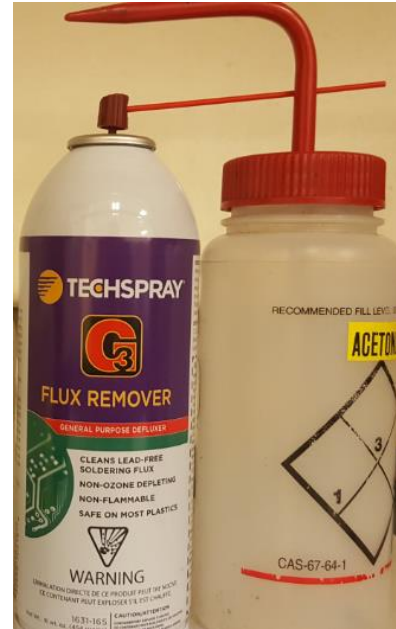
Figure 12-1: examples of acetone and flux remover which can be used to remove flux
