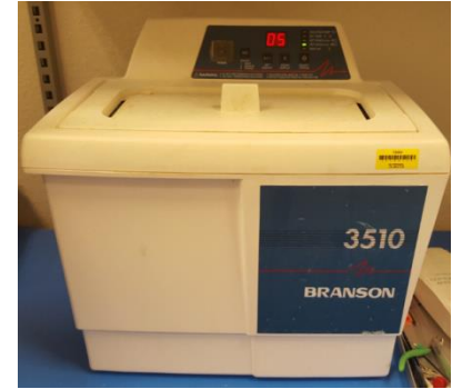
Figure: 12-2 An example sonic bath tool, Branson 3510
