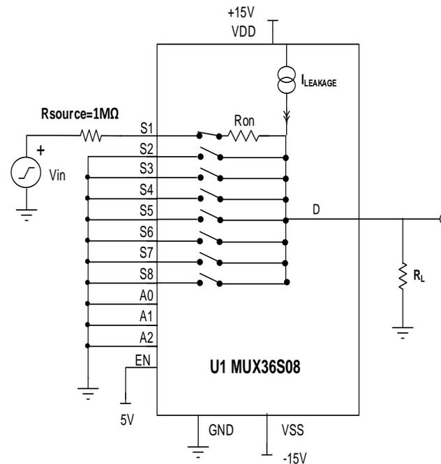
**2. There is an option to select one of the two multiplexers (MUX1 and MUX2) for a given DAQ system. MUX1 and MUX2 have charge injection figures of 1pC and 4.7pC respectively. MUX1 has an output load capacitance of 47pF while MUX2 has a load capacitance of 100pF. Which multiplexer will have minimum voltage error due to charge injection at the output?**
